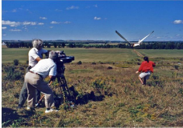
Mr. Bill on his way -- the twisting of the shear, flexing wings is clearly visible
