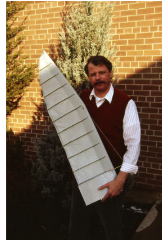
Jim at UTIAS with completed Greywing outer panel, showing exposed ribs on its upper surface
