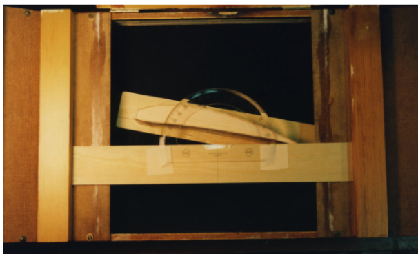
Adjusting the angle of an airfoil model in the test section of the "two-dimensional" tunnel
